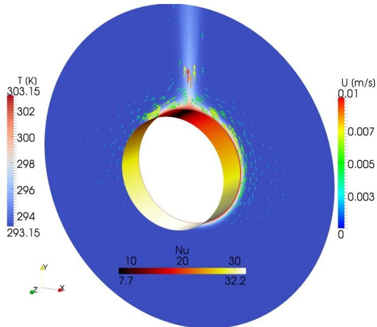
**Figure 3: Visualisation of the flow separation and recombination around the cylinders circumference, the temperature field and the local Nusselt number for a cylinder with diameter 35mm and  $\Delta T = 10\text{K}$ .**
