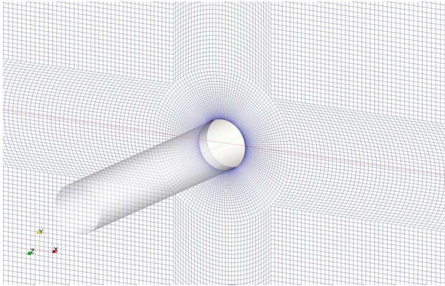
Figure 1: A trimetric view of the hexahedral mesh<sup>2</sup> around the cylinder (parameterised with Gmsh<sup>3</sup>).
