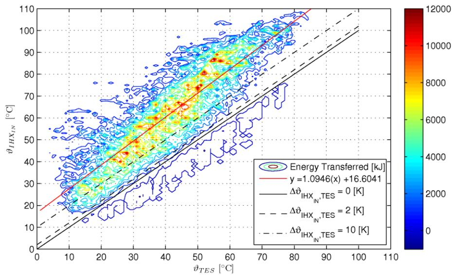
Figure 7. Energy weighted temperature histogram for  $\dot{m} = 10 \text{ kg} / \text{h.m}^2$  collector area;  $\Delta\vartheta_{\text{IHX}_{\text{IN}}, \text{TES}}$  is 10 K for switching on and 2 K for switching off.
