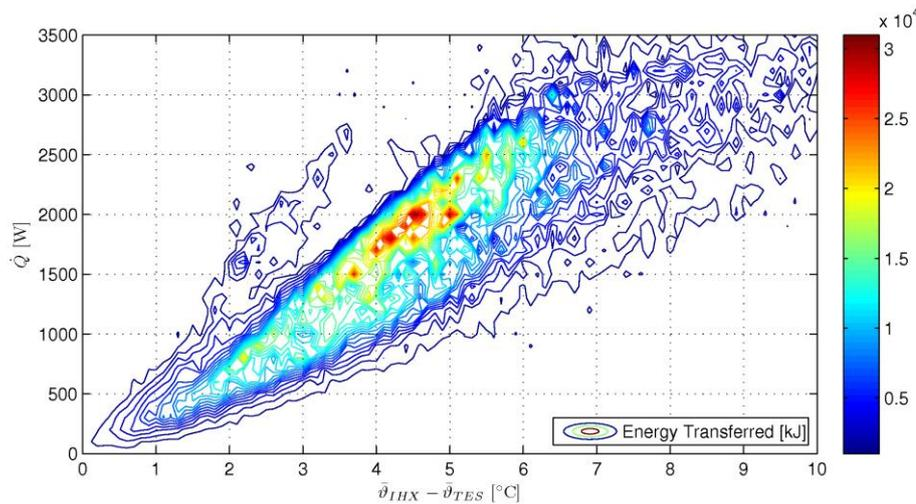
Figure 6. Collector power as a function of *mean temperature difference* between IHX and TES for  $\dot{m} = 10\text{kg} / \text{h.m}^2$ .
