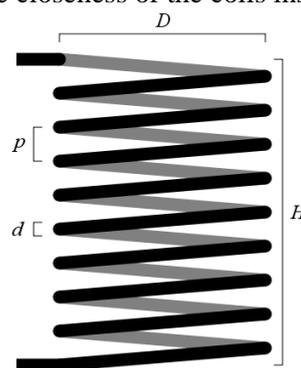
Figure 1. Cardinal geometrical parameters of an IHX. Through mathematical simplification we can sketch such a helixed tube in cartesian coordinates by rotating a circle around the helixes centre with a pitch  $p$  climbing the  $z$ -axis. When we speak of the  $p/d$  ratio though, we subtract  $d$  from  $p$  such that only the distance between coils is implied; which then coincides with common nomenclature.
