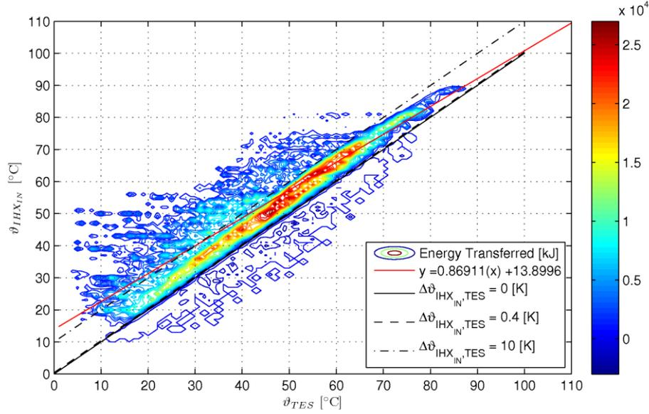
Figure 8. Energy weighted temperature histogram for  $\dot{m} = 50 \text{ kg} / \text{h.m}^2$  collector area;  $\Delta\vartheta_{IHX_{IN},TES}$  is 10 K for switching on and 0.4 K for switching off.
