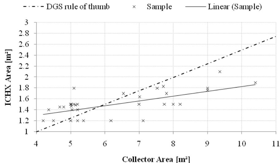
Figure 4. A sample of 38 solar thermal packaged systems showing the relationship of collector area to IHX surface area.
